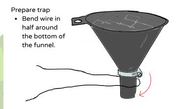
• Twist wire ends for ~5 cm, so the twisted part sticks out as far as the funnel's tab. The loose ends will be attached to the support.
